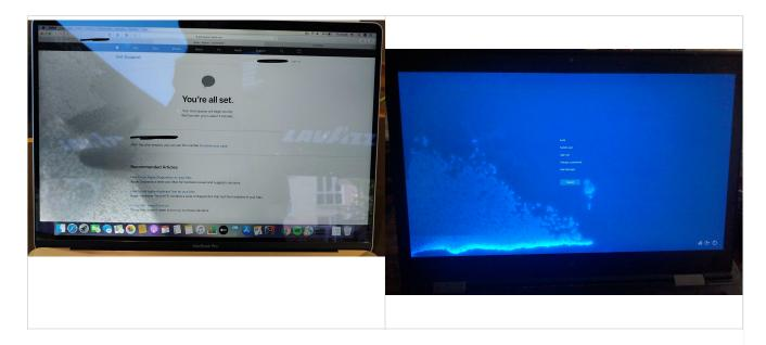
Liquid damage is one of the most common and **harmful** issues to befall an electronic device. It can happen **directly** (e.g., spilling a liquid on the device chassis) or **indirectly** (e.g., storage in a humid environment).
