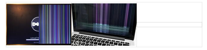
Laptop and phone displays are **fragile** and prone to cracking, especially when subjected to **sudden force** (e.g., a drop) or **sustained pressure** (e.g., between or underneath heavy books in a backpack).
