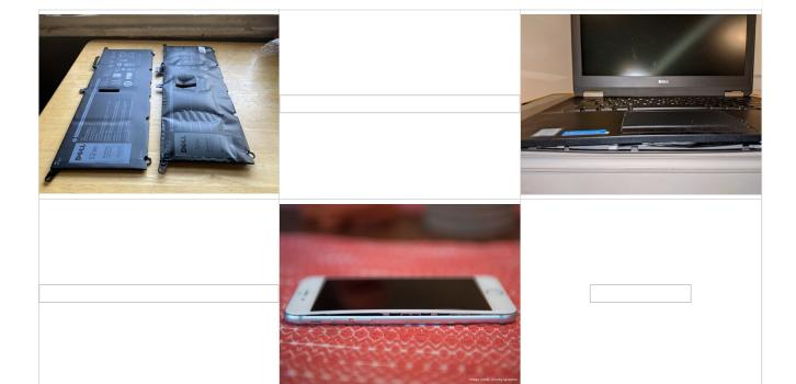
Batteries slowly change shape over their lifespan, but this process can be worsened through bad charging habits or a poor quality battery. Check the frame of your laptop or phone for signs of **warping** -- try placing the device on a flat surface and **see if it is wobbly or unbalanced**.
