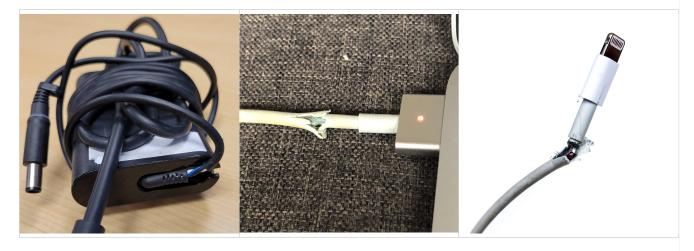
The shielding around modern cables can withstand a fair amount of wear and tear. However, bending the cable or wrapping it tightly can cause specific "joints" in the cable to wear out more quickly and potentially **break the shielding** or the **cabling** itself.
